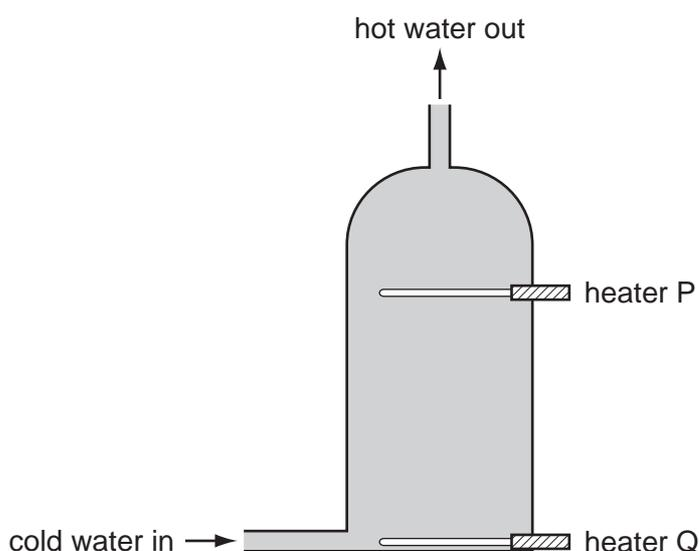
When only heater Q is switched on, it takes a very long time to heat the tank of water to the required temperature of  $60^{\circ}\text{C}$ .
